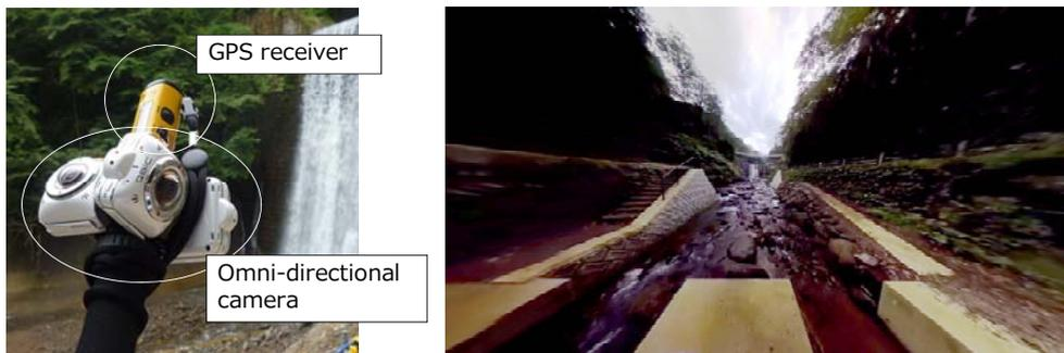
**Figure 5.** A GPS mounted omni-directional camera (left image) and captured movie with position and rotation data (right image)
