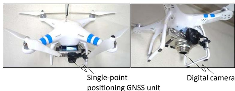
**Figure 3.** Small UAV with compact digital camera and GPS unit.
